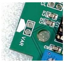
On the PCB you will see a two pin rectangle marked VAR. This is where the varicap diode must be fitted, by the rectangle the outline shape is
