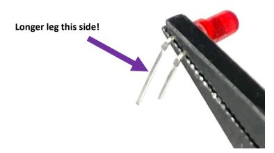
The best way to fit the led at the correct hight is to temporally fit the front panel. Only loose at this point. Drop the LED into place (again make sure the long leg side is nearest to the switch) and pop the front panel in place, I tend to tighten the bandwidth nut a little by hand to hold it in place. Then carefully position the LED so it protrudes through its mounting hole and sits at the correct hight, turn the board over and solder the LED pins in place.
