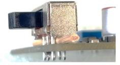
When you are happy that it's sat correctly solder the remaining pins. When finished pull out the stick.
